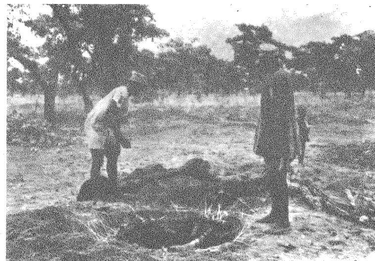
Plate XII Tiza; charcoal-making. Logs being placed in a pit.
