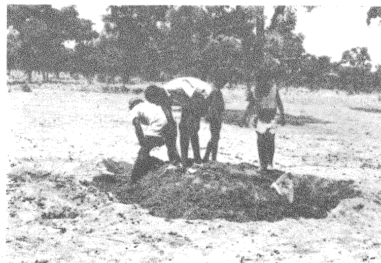
Plate XIII Tiza; charcoal-making. Logs burning and covered with earth.
